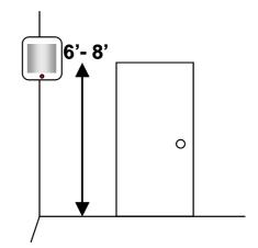
person sitting in front of a computer or reading in a comfortable chair will not be moving enough for EZMotion to detect unless it is placed close to the person. The sensitivity of EZMotion can be set to high or the time delay when lights are turned off can be made fairly large (1 hour or more) to compensate for situations where people are sitting still. The best location is usually in the corner of the room adjacent to the entry door.
